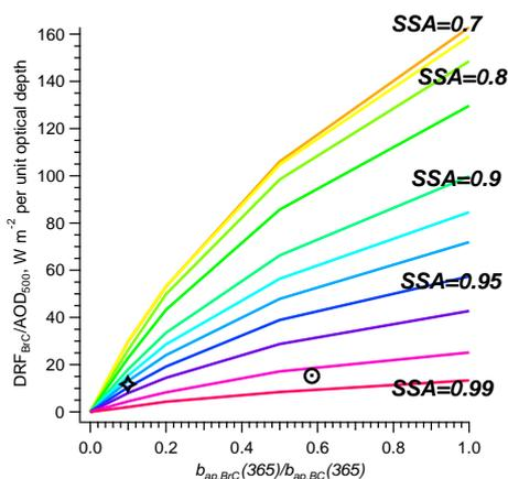
**Figure 10.** BrC radiative forcing efficiencies, defined as the BrC TOA direct radiative forcing divided by AOD at 500 nm, as a function of BrC to BC absorption ratio and SSA measured at surface at 365 nm. The circle corresponds to average background conditions determined from the DC3 campaign. The star represents a surface measurement from southeast USA, where altitude-resolved data were not available.
