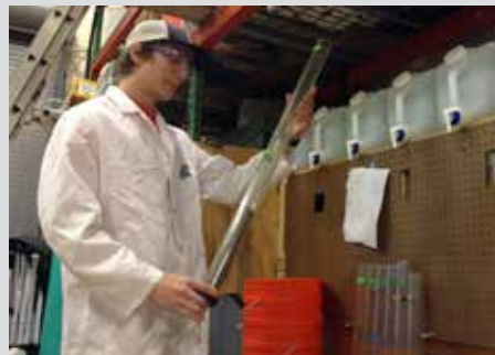
We used controlled column studies to explore how different soil gradients, depths, and amendments perform with respect to phosphorus removal from typical urban stormwater runoff. Column studies are a quick, efficient way to test the performance of a wide range of filter media.
