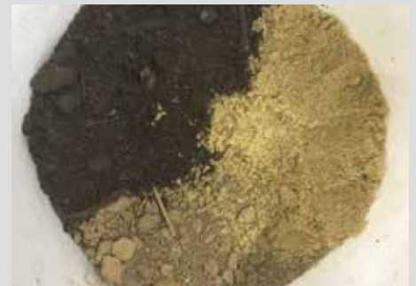
Sand, loam, wood chips, and compost are common components of filter media. Research has shown that compost can be a source of phosphorus and therefore is no longer recommended. Coconut coir fibers or peat moss are suitable substitutes.
