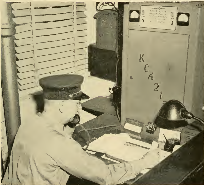
The new Fire Department FM radio provides two-way communication between the Lakeport, Weirs, and Central Station, with one fire truck at each station, and with the Chief's car.
