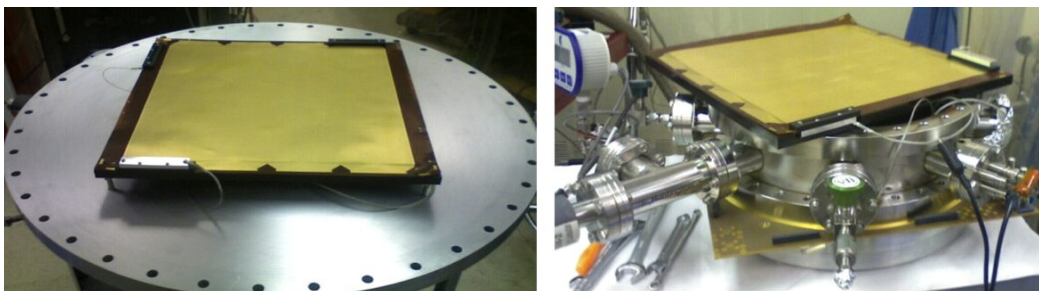
Figure 7 – Assembly of the 30 cm prototype hardware. The 30×30 cm 2 MWD is visible on top of parts of the gas pressure chamber.
