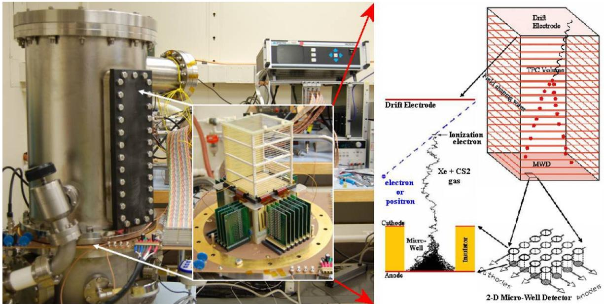
Figure 1  $\sim 10 \times 10 \times 15$  cm<sup>3</sup> 3-DTI prototype (inset photo) and vacuum chamber (left). Schematic diagram of the 3-DTI TPC, MWD and simulation of an electron induced avalanche in a micro-well (right).
