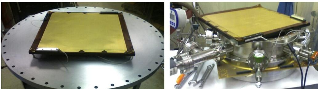
Figure 7 – Assembly of the 30 cm prototype hardware. The 30×30 cm<sup>2</sup> MWD is visible on top of parts of the gas pressure chamber.
