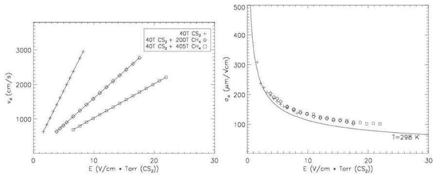
Figure 5 – The negative ion drift velocity in CS<sub>2</sub> at 40 torr and CH<sub>4</sub> at 0, 200, and 400 torr as a function of the reduced field (*left*). The solid lines are linear fits to the data points. The longitudinal diffusion for the same gas mixtures as a function of reduced field (*right*). The solid line is the thermal diffusion expected at 298 K. The symbols used in the two plots correspond to the same CH<sub>4</sub> pressures.
