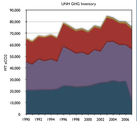
The superior efficiency of the plant, its use of less carbon intensive fuels like distillate (#4) fuel oil or natural gas instead of carbon intensive residual (#6) fuel oil, and the subsequent reduction in electricity needed to be purchased have lead to significant reductions in overall UNH emissions.
