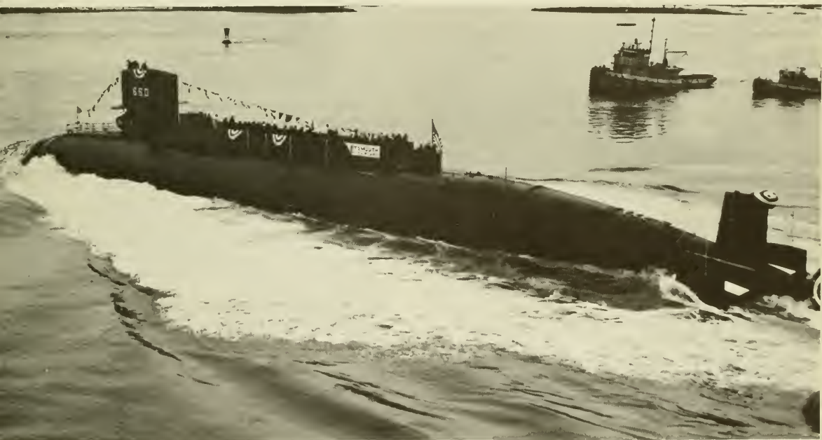
SSN 660 (SAND LANCE) Keel laid 15 January 1965 Launched 11 November 1969 A nuclear attack submarine with a 292 foot length and a displacement of 4,600 tons submerged.
