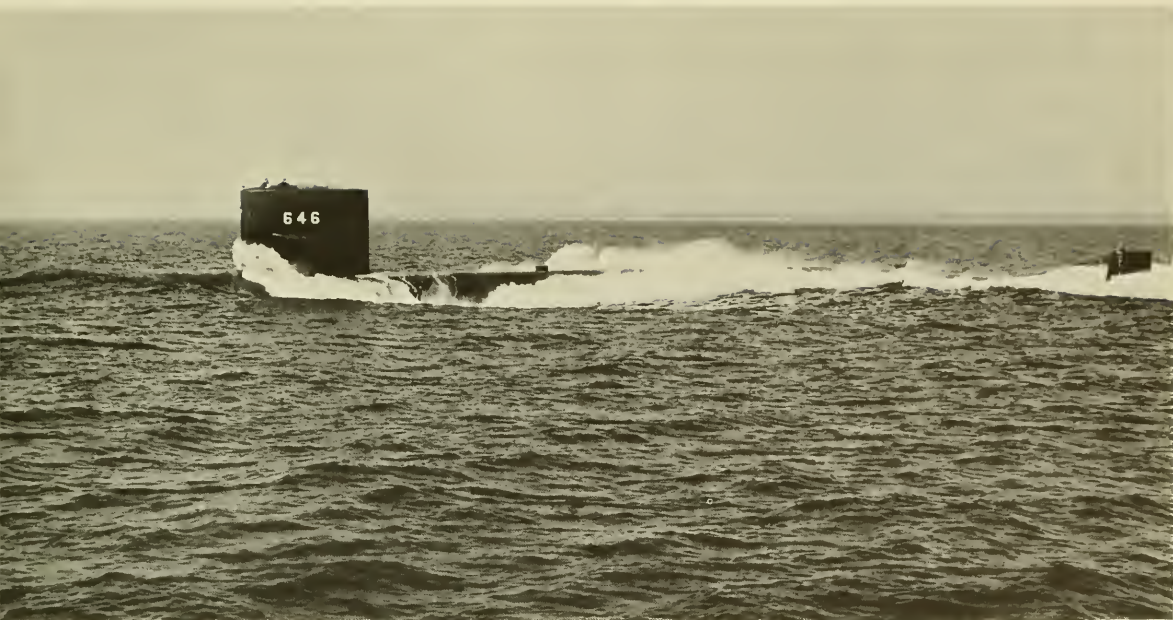
USS GRAYLING (SSN 646) Keel laid 12 May 1964 Launched 22 June 1967 Commissioned 11 October 1969 A nuclear attack submarine with a 292 foot length and a displacement of 4,600 tons submerged.
