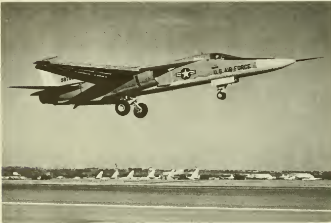
FB-111 STRATEGIC BOMBER — The FB-111 will be entering the Strategic Air Command inventory during 1970, and a number of the aircraft are scheduled to be stationed at Pease Air Force Base. The wings of the FB-111 can be varied in flight to provide stable and efficient performance. The FB-111's will be replacing the B-52's which departed Pease in November, 1969.
