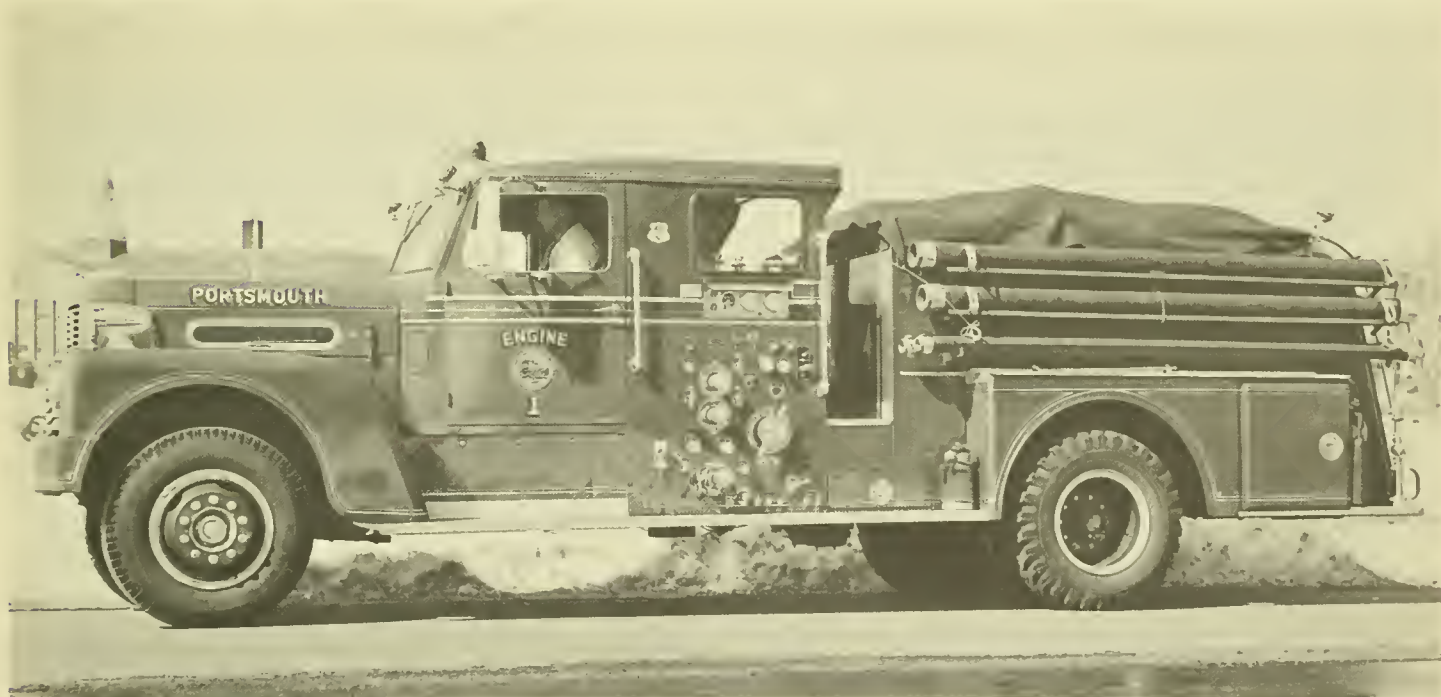
Central Fire Station New Howe Pumper -750 gallons
