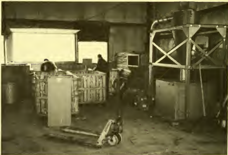
Town employees sort materials at the Recycling Center. Plastic granulator at right.
