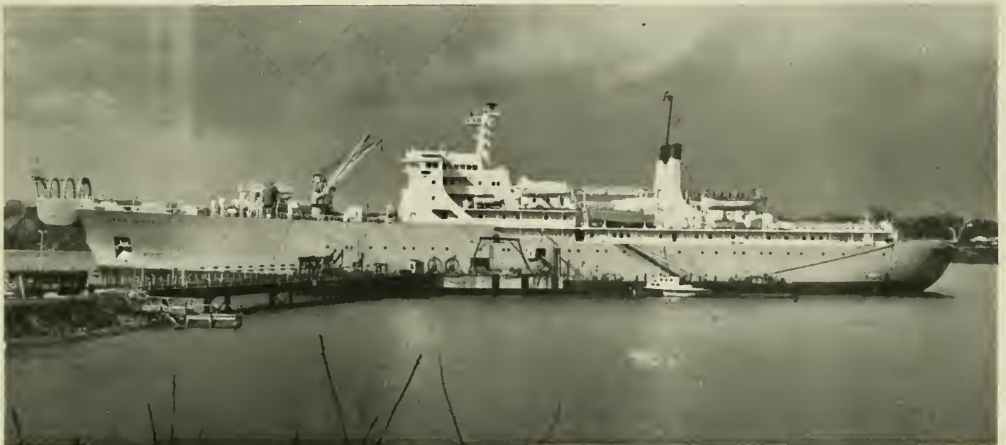
Cable ship "Long Lines" owned by Transoceanic Cable Company, a subsidiary of American Telegraph & Telephone Co. Moored at Simplex Wire & Cable Company plant in Newington, N. H. on her maiden voyage for first consignment of cable. Built in West Germany the "Long Lines" will lay the first direct telephone cable between the United States and Europe.
