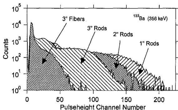
Figure 11: Spectra from  $^{133}\text{Ba}$  recorded for different scintillator assemblies (of varying lengths) and for a scintillating fiber bundle. In all cases, the individual elements (or fibers) were  $5 \times 5 \text{ mm}^2$ . The relative light output of the scintillator assemblies is clearly superior to that of the scintillating fibers.
