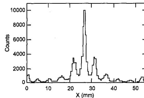
Figure 10: Distribution of events in the fiber bundle when irradiated with a collimated beam of 662 keV photons from <sup>137</sup>Cs. (Beam spot size ~3-4 mm.)
