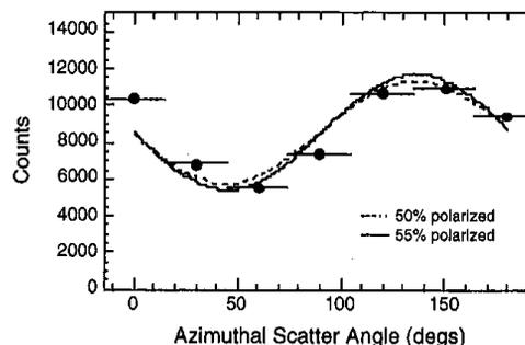
Figure 3: The prototype response to a polarized beam incident on-axis, but with a polarization angle rotated  $-45^\circ$  with respect to that in Figure 4. The smooth curves represent simulation results.
