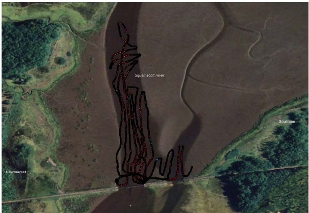
Figure 5. Squamscott River post-construction video results showing ship-tracks and shell areas
