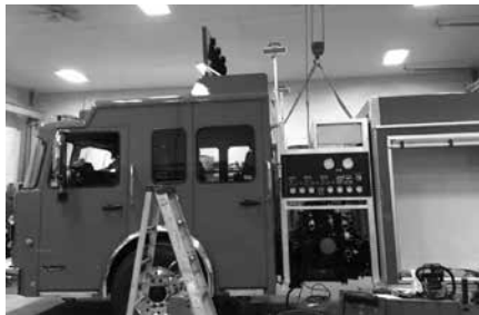
Cabinet doors and pump panel installed
