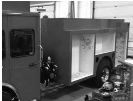
The body and pump mounted to the chasis.
