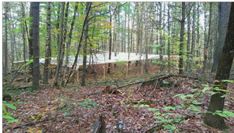
The Thompson Farm throughfall manipulation structure on one of the treatment plots designed to remove 55 percent of incoming precipitation. Photo by David Sims, UNH-EOS.
