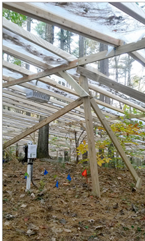
Series of parallel troughs capture rainfall and funnel it away from the treatment plots where it can be measured and diverted.
