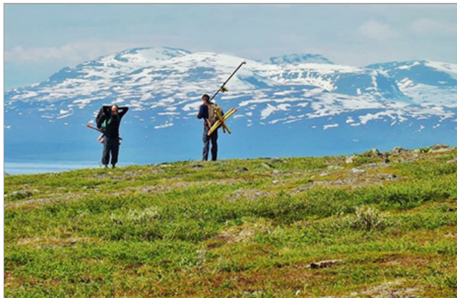
The uplands of Vassijaure, Sweden west of Abisko. Mike Palace (left) and Kellen McArthur collect photographs using the drone. Palace carries on his back. The yellow Xs McArthur holds were placed on the ground and used as control points for the drone imagery and referenced using the GPS unit also carried by McArthur. Photo by Jessica DelGreco, UNH-EOS.
