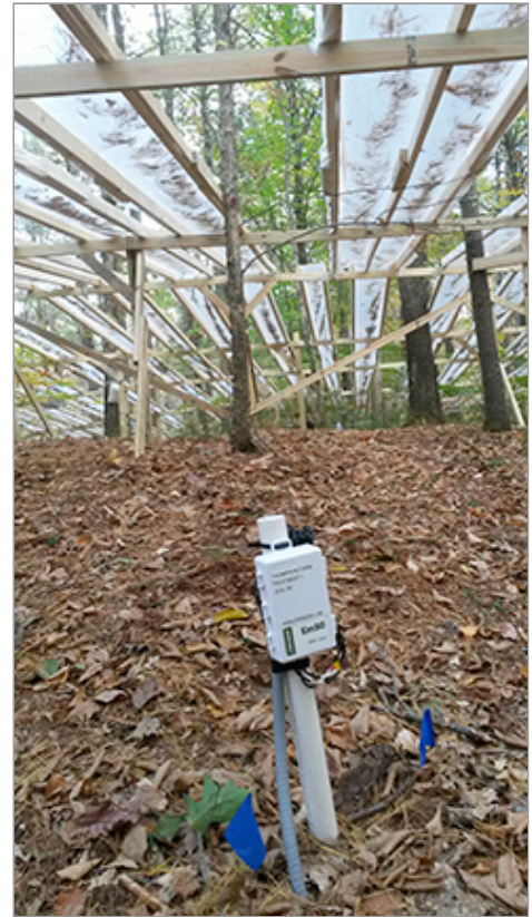
A data logger used for soil moisture sensors mounted in the foreground. Volumetric water content and soil temperature will be recorded at multiple depths every 15 minutes throughout the four-year study period. Photo by David Sims, UNH-EOS.
