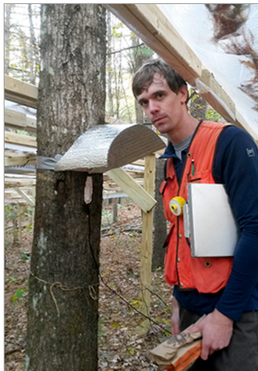
Ph.D. student Cameron McIntire checks on a soil moisture sensor modified to measure sapwood water content in a northern red oak. Photo by David Sims, UNH-EOS.
