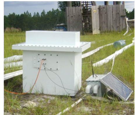
The x-ray instrument pictured in the foreground was the first instrument used to record x-rays from rocket-triggered lightning. In 2002, measurements made by this instrument established that lightning emits bright bursts of x-rays, giving researchers a new tool for studying lightning. Photo courtesy of Joseph Dwyer, UNH-EOS.
