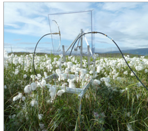
An automated chamber system used to measure methane emissions from Methanoflorens stordalenmirensis, the previously unknown species of microbe that McCalley and colleagues discovered in Stordalen Mire, Sweden. Photo by Carrie McCalley, UNH-EOS.
