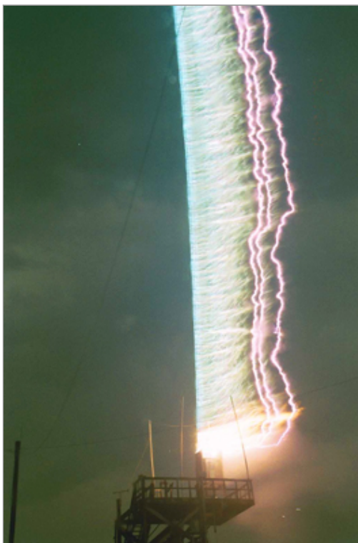
Rocket-triggered lightning was found to generate x-rays, providing clues to how lightning propagates to the ground. The top of the rocket launch tower is at the bottom of the picture. Photo courtesy the University of Florida.
