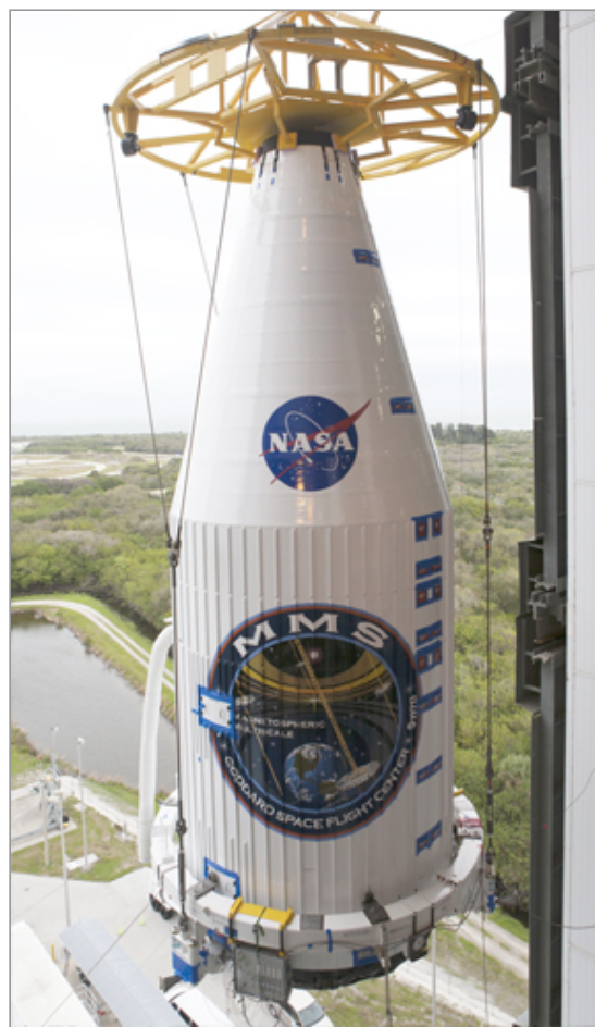
The MMS payload in the process of being lifted onto the Atlas V rocket at the Cape Canaveral Air Force Station Vehicle Integration Facility. Photo courtesy of NASA.
