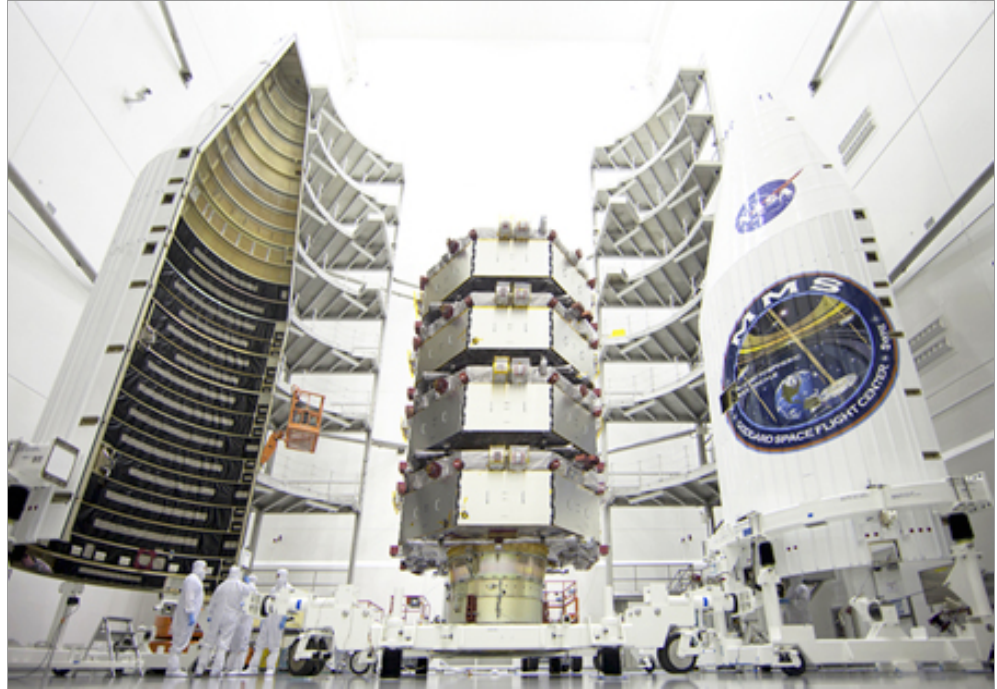
The stacked MMS spacecraft being encapsulated in the payload fairing. Photo courtesy of NASA.
