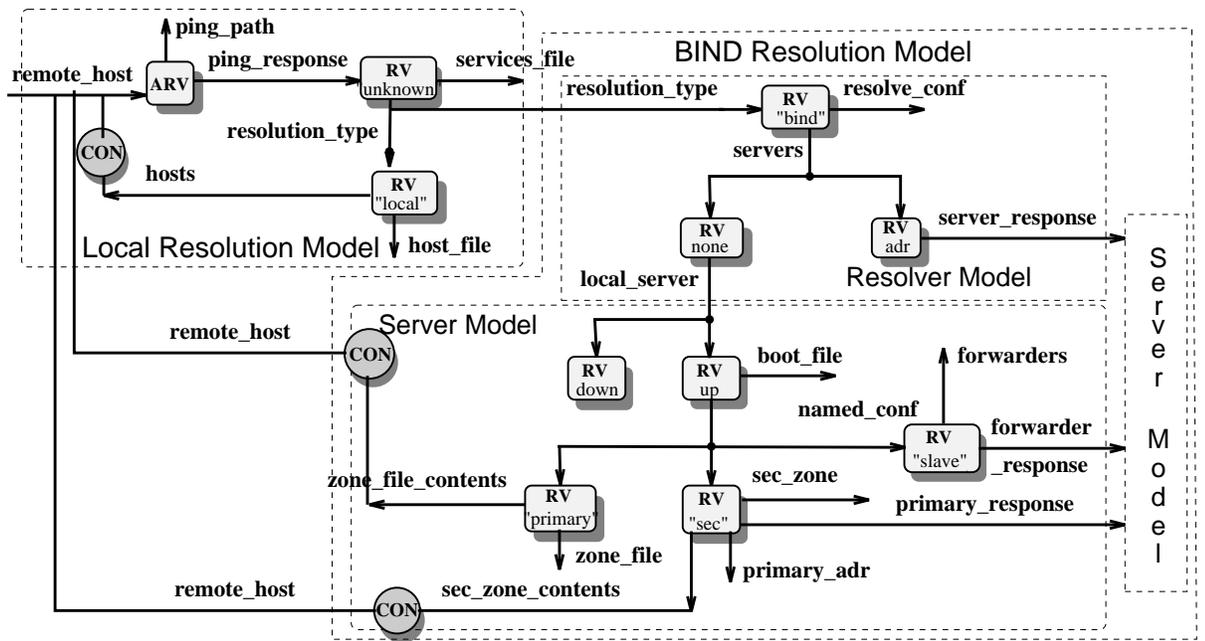
Figure 6 DNS configuration model formulated as a DCSP
