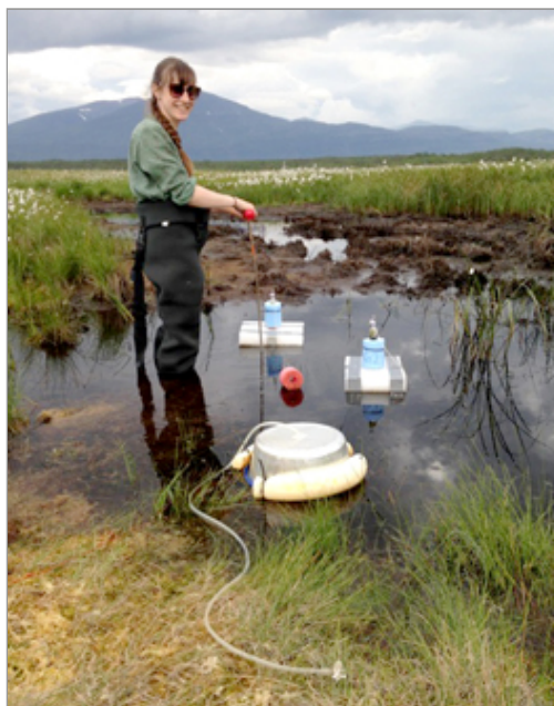
Sophie Burke deploys two UNH-developed methane traps in thaw ponds at the Stordalen Mire research site in Abisko, Sweden. The measurements are helping to quantify the powerful greenhouse gas's global budget. Photo by Justine Ramage, Stockholm University.
