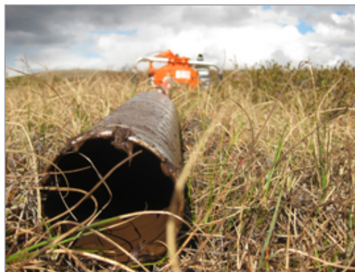
Gas-powered auger with a peat corer barrel attached.
