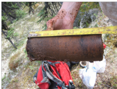
Treat holds a 20-centimeter core drilled from a site with intact permafrost in the Innoko NWR.
