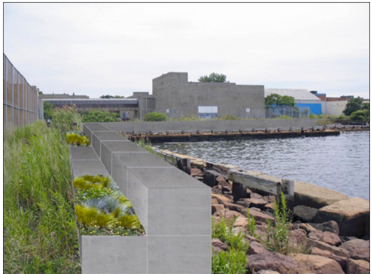
Conceptual design of a modular floodwall that can be increased in size as needed due to sea level rise. Image prepared by the Woods Hole Group, Inc. for a NOAA-funded UMass-Boston, UNH, UMD project "Coastal Flooding and Environmental Justice: Developing Strategies for Adapting to Climate Change." Courtesy of Paul Kirshen, UNH-EOS/CE
