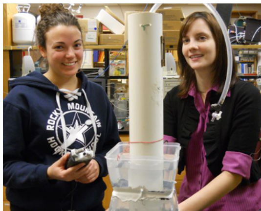
Undergraduate Jacki Amante (left) and Jillian Lennartz conduct calibration tests on the hydrophone-based ebullition instrument invented at UNH.
