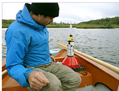
Martin Wik, a graduate student at Stockholm University, installs bubble sensors in Mellan Harsjön, a lake adjacent to Stordalen mire. Photo by Ruth Varner, UNH-EOS.
