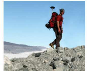
Ryan Cassotto conducts a GPS survey to profile a lateral moraine above the researcher's camp at Kangiata Nunata Sermia. The moraine (debris in foreground) represents the maximum extent of the last major glacial advance during the Little Ice Age. Photo by Mark Fahnestock.
