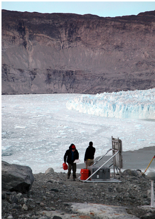
Two collaborators from the University of Alaska Fairbanks at the terminus of the glacier. Also pictured are a solar panel and battery bank that power year-round GPS observations, used by the researchers to measure uplift of the area in response to the loss of ice. Photo by Mark Fahnestock.
