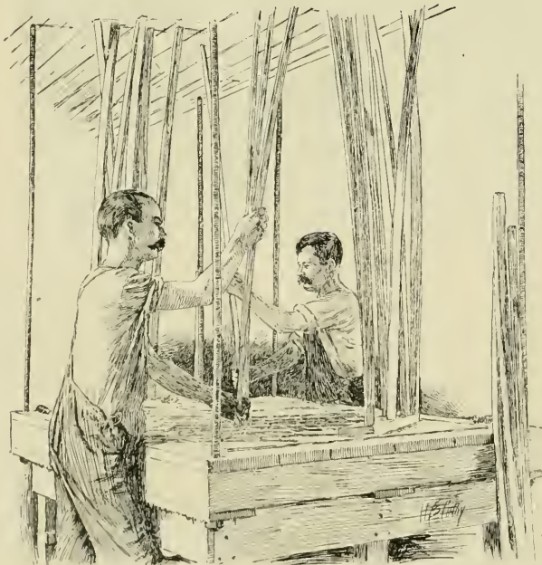
Gluing Bars on the Sounding-Board.
