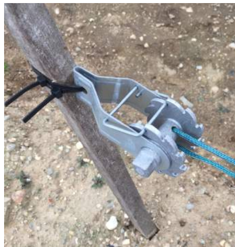
Fig. 24: Tensioner installed on a wooden tomato stake. Photo: K. Orde
