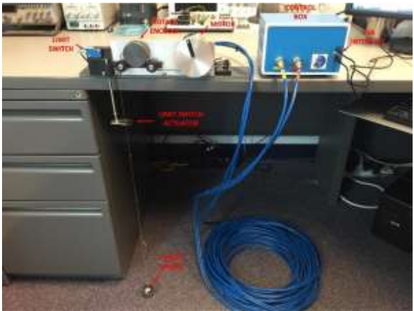
Figure 3.1. Upgraded vertical target positioning system on bench
