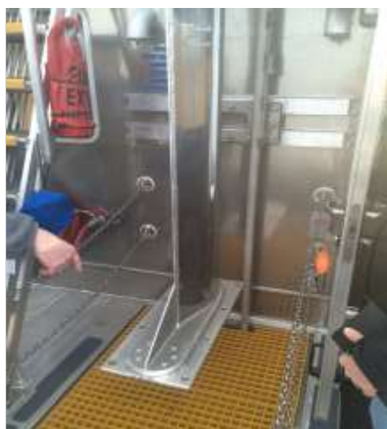
Figure 1-9: Bottom of 3.5m long hydraulic ram for mounting sonars and deploying through moon pool (covered by yellow grating) on R/V Gulf Surveyor .
