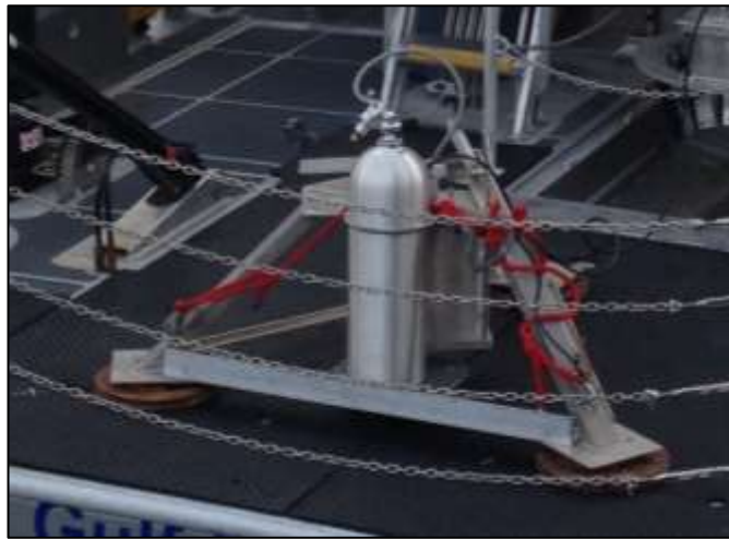
Figure 5-31: A synthetic air bubble seep generator ready for deployment on the R/V Gulf Surveyor.
