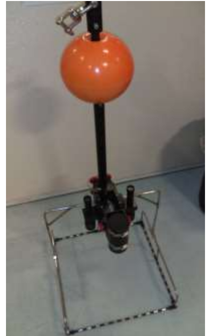
Figure 5-25: Second generation Imaging Grab Sampler. Left – with Pohner corer, Right – standing.
