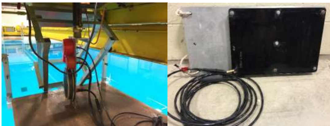
Figure 3-2. Some of the transducers tested in the acoustic tank in 2016. Left: Simrad ES120 and 200 and MSI Constant Beamwidth Transducer; Right: Edgetech PVDF transducer.
