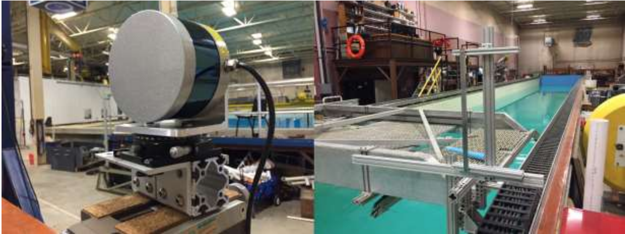
Figure 3-11: Left: Laser scanner mounted vertically centered over the ultra-high precision rotating compass. Right: Narrow vertical aluminum target.
