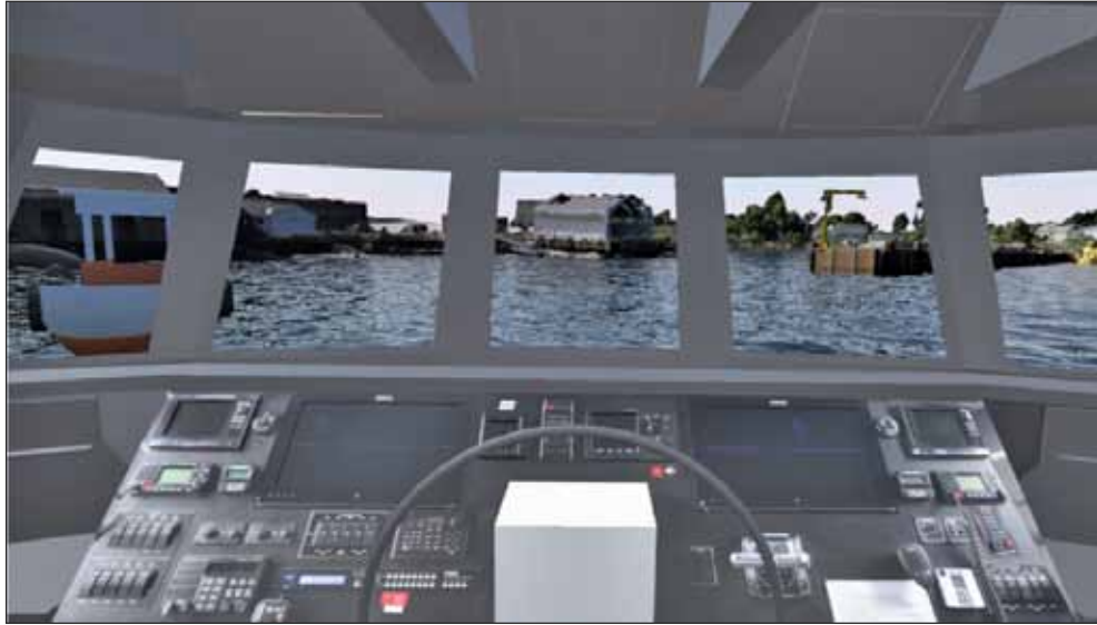
Figure ES-30. Screenshot from within simulator, showing view from inside virtual Gulf Surveyor's bridge, with photo-textured instrument panel, looking towards UNH's New Castle Pier.
