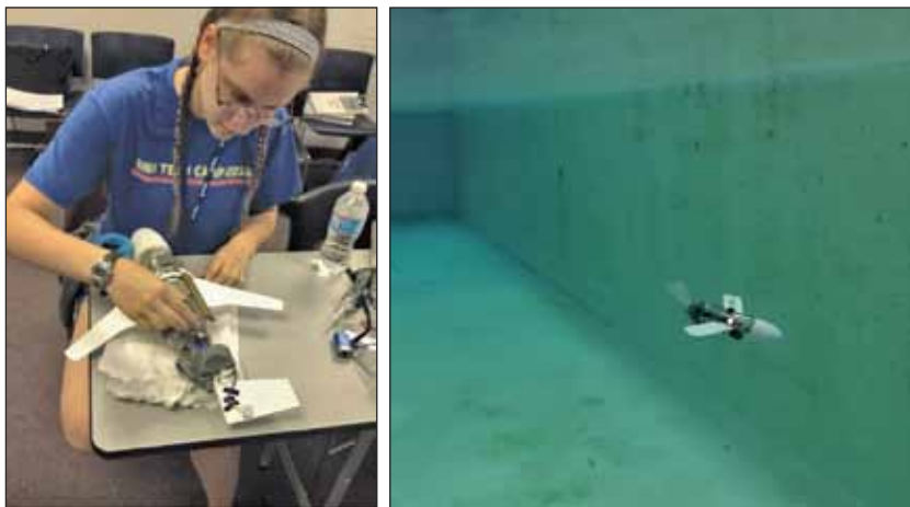
Figure ES-40. Advanced Tech Camp attendees building a SeaGlider—a small autonomous underwater buoyancy-driven vehicle.
