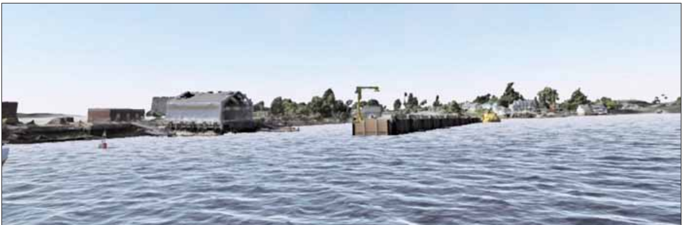
Figure ES-31. Panoramic screenshot from inside the AR simulator showing realistic (and changeable) ocean model and the coast line features generated through Structure from Motion process using a 394-photo dataset.
