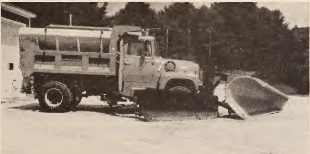
Truck for Highway Department, with equipment: sander body, snow plow and wing.
