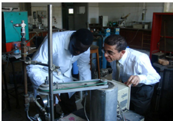
Emmanuel Pitia and Professor Farag at the NRC lab looking at the meter of a high pressure reactor. The reactor is used for producing biodiesel via supercritical methanol method.
