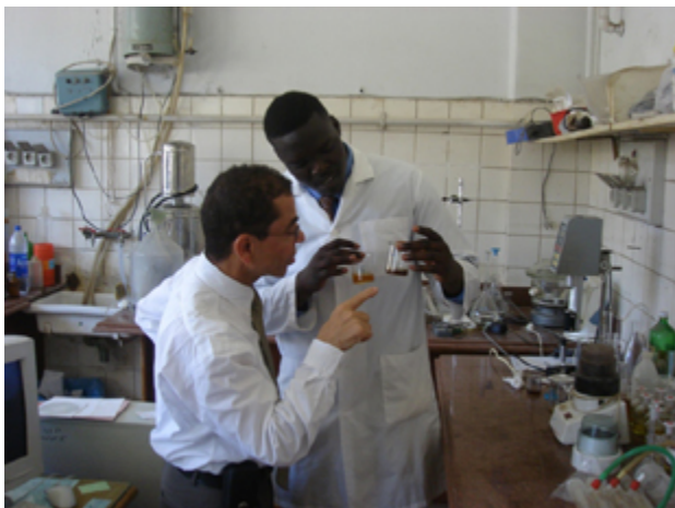
Emmanuel Pitia and Professor Farag at the National Research Centre lab in Cairo, Egypt, comparing the color and flow of oil extracted from jatropha using Hexane (yellowish sample) and isopropanol (dark sample) as solvents.
