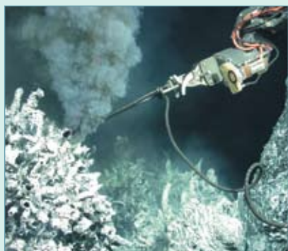
The arm of the remotely operated vehicle (ROV) Jason II measures the temperature of the newly discovered Medusa hydrothermal vent.
