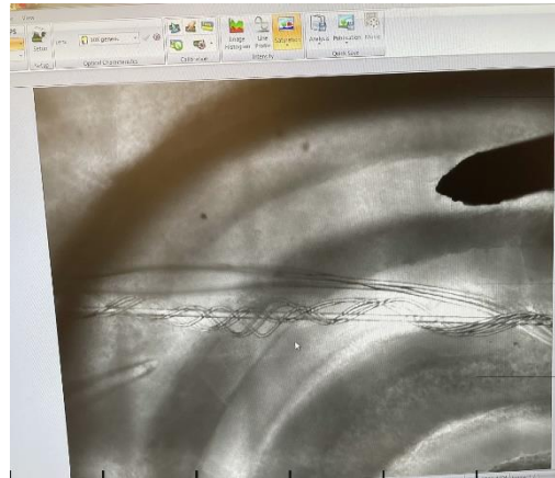
A microscope image displayed on a computer screen showing a mouse hippocampal brain slice with stimulus and recording electrodes inserted in it.
