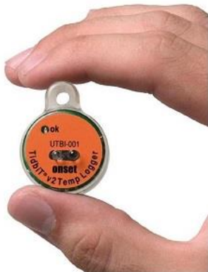
Figure 2. HOBOWare Tidbit v2 Water Temperature Data Logger size in relation to a hand. (Photo by Onsetcomp.com.)
