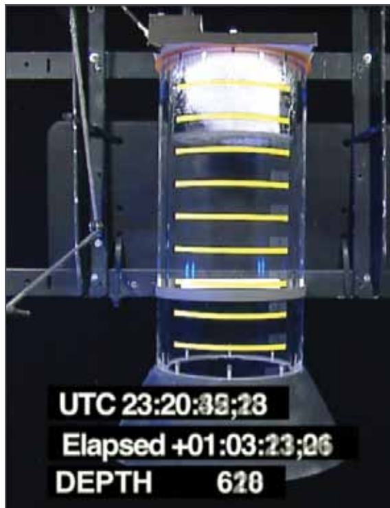
Figure ES-9. A methane capture device used to assess methane flux from a seep in the Gulf of Mexico. Note the hydrates forming in the top of the cylinder, which dissociate to form gas and water as the ROV rises to shallower depths and warmer waters.
