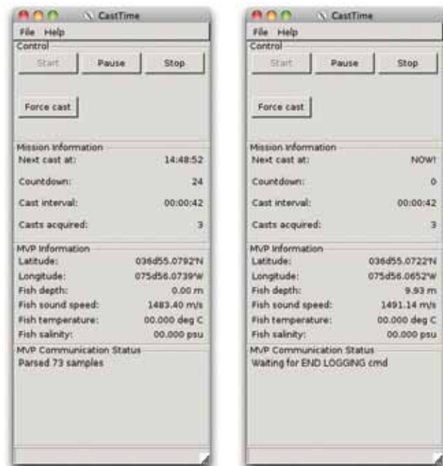
Figure 3-16. Early version of the CastTime graphical user interface showing countdown and casting modes (left and right, respectively).
