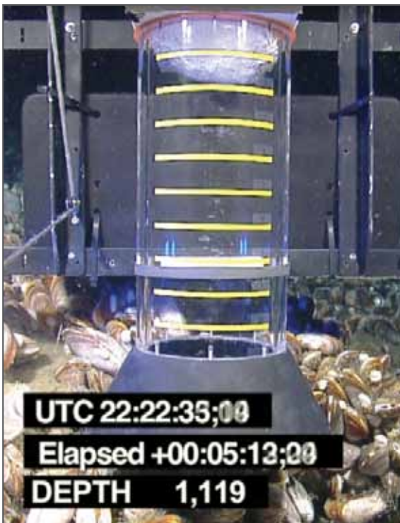
Figure ES-9. A methane capture device used to assess methane flux from a seep in the Gulf of Mexico. Note the hydrates forming in the top of the cylinder, which dissociate to form gas and water as the ROV rises to shallower depths and warmer waters.
