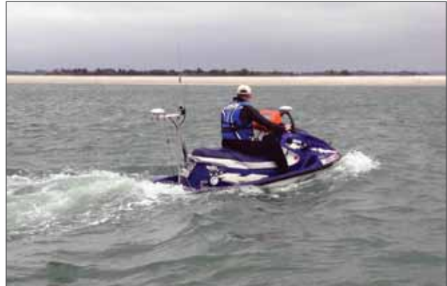
Figure 3-5. Photograph of the CBASS in operation at the RIVET field experiment at New River Inlet, NC.
