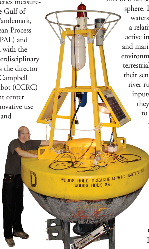
Doug Vandemark readies the buoy that will measure coastal ocean carbon dioxide levels for the first time in the Gulf of Maine.
