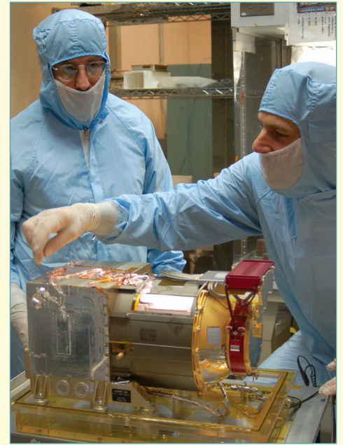
John Gaidos, left, and Stan Ellis benchtest PLASTIC Flight Model No. 1
