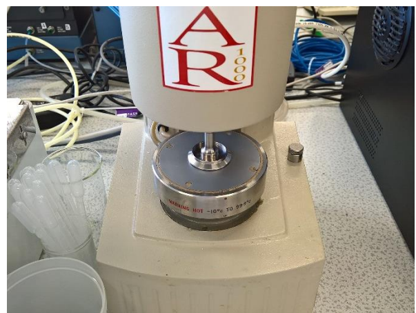
Figure 2. A rheometer shows the metal plate fully lowered down on top of the stage. The hydrogel was placed between the metal plate and stage to test stiffness. (Photo copyright 2016 Nick Birse, Wikimedia Commons, "TA Instruments AR1000 Rheometer.")
