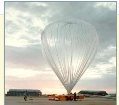
A balloon like this, thinner than a garbage bag and filled with six million cubic feet of helium, will haul the 2.5 ton BalloonWinds payload aloft to 100,000 ft.
