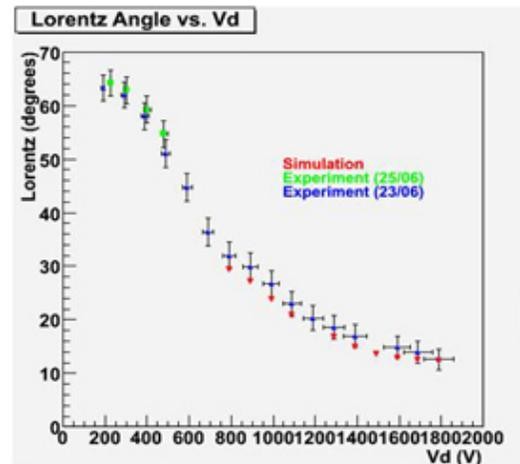
To determine the Lorentz angle, we used data from the readout electronics to calculate the position of the voltage spike, which represents the location where the photons entered the detector. We also determined the center of the broader distribution of voltage spikes that appears next to the initial spike and represents the electrons' positions as they drifted across the detector (Fig. 5). We used the distance between these two positions to calculate the Lorentz angle.
