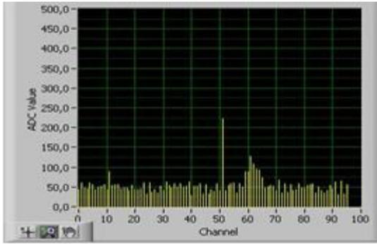
LEFT: Fig. 6 – Example of data output from Micromegas detector electronics. Seen here is the sharp peak from the laser (left) and the drifted electrons (right) (5)
