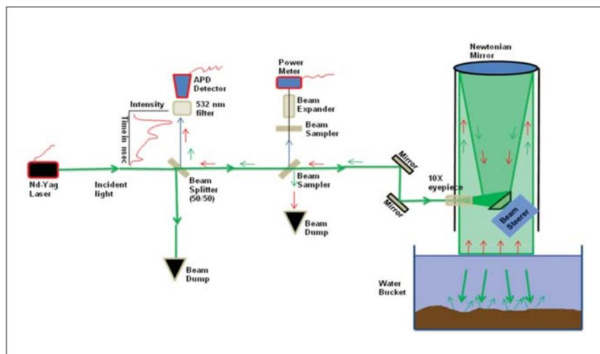
Figure 2. Schematic illustration of the bathymetric LIDAR simulator.
