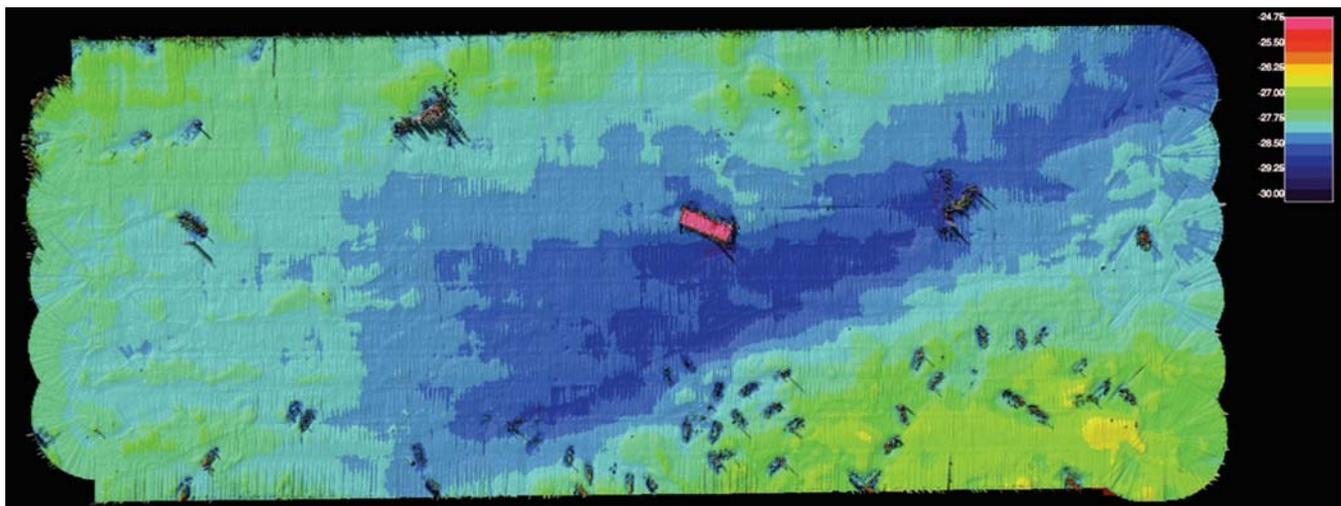
Figure 45. "Redbird" survey site off the Delaware coast in which several sunken subway cars, a shipwreck and a sunken barge are clearly evident.
