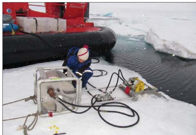
Figure 18. Hydrostatic corer being tested from Hovercraft *Sabvabaa*.
