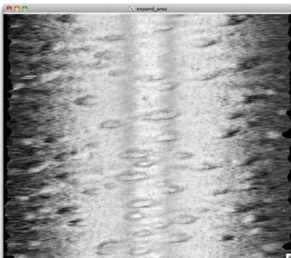
Figure 46. Waterfall display of “intensity” seabed imagery data.
