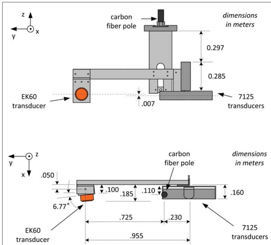
Figure 27. Test mounting for sonar calibration trials.
