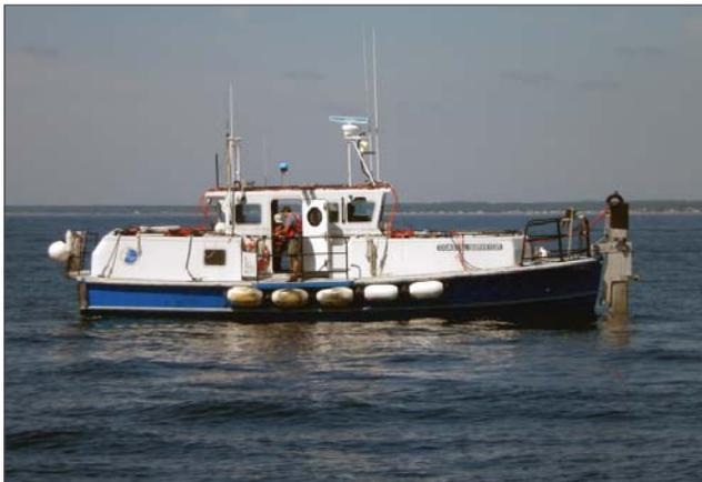
Figure 15. R/V *Coastal Surveyor* with bow ram.
