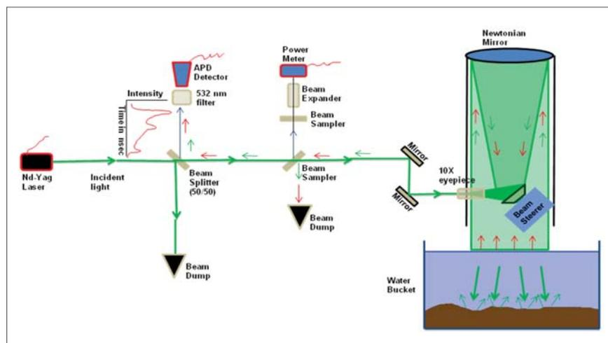
Figure 68. Schematic illustration of the bathymetric lidar simulator.
