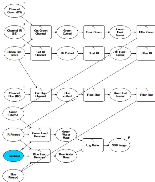
**Figure 1.** SDB toolbox used in *ArcMap*.
