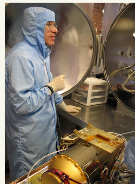
STEREO-PLASTIC co-investigator Mark Popecki tests Flight Model #2 in the Morse Hall vacuum chamber.
