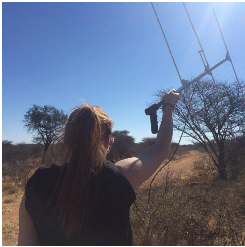
The author using an antenna cabled to a receiver to track signals from the cheetah Zinzi’s radio collar—a basic method for tracking wild animals using radio telemetry.
