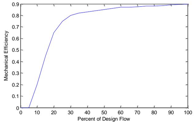
Fig. 6. Mechanical efficiency of the Archimedean Screw vs. flow rate.
