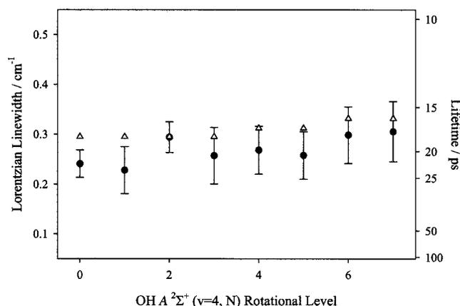
FIG. 4. Linewidths and corresponding lifetimes of OH  $A\ 2\Sigma^+$  ( $v=4, N$ ) rotational levels derived from the Lorentzian component of FDIR line profiles (filled circles) and first-principles theory (open triangles; Ref. 1). The linewidths are nearly invariant over the range of rotational levels examined.
