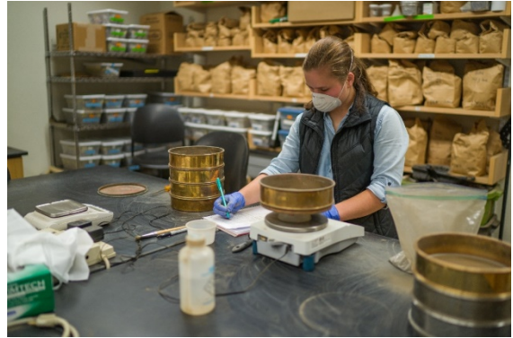
The author conducting sieve analysis on sediment samples. Photo credit: Jeremy Gasowski.
