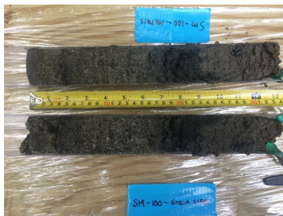
Sediment core collected at Sawyer Mill impoundment using a gravity corer.
