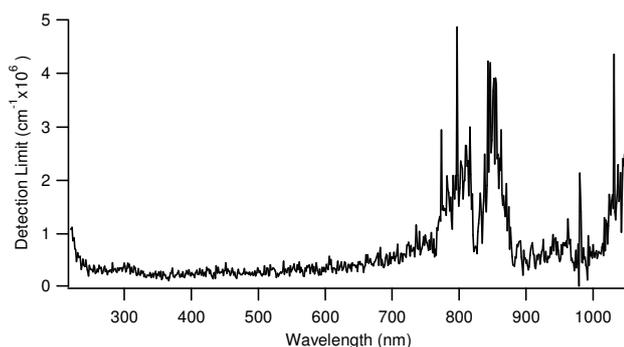
**Fig. 3.** The AE-DOAS detection limit is shown as a function of wavelength. This data is smoothed by averaging over five recorded wavelength values. It is clear that the detection limit is steady over the center of the solar spectrum from 235–700 nm. At wavelengths outside this range, the detection limit increases due to low lamp intensity and is not used in our experiments.
