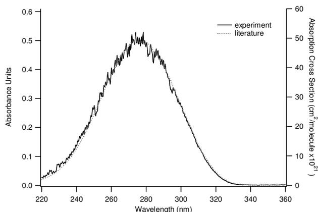
**Fig. 6.** The UV absorption spectrum obtained with the AE-DOAS of acetone with a 5-point boxcar average is shown as a solid black line. This is compared with the dotted grey line showing the absorption cross section spectrum of gas phase acetone (shown on the right y-axis) (Meyrahn et al., 1986).
