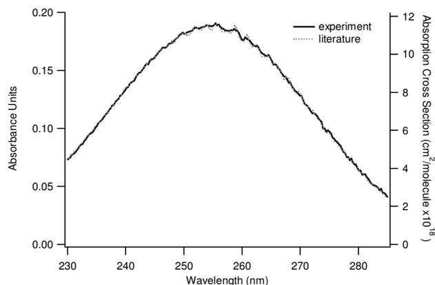
**Fig. 5.** The UV absorption spectrum of the Hartley band of ozone measured with an AE-DOAS path length of 9.75 m is shown as a solid black line. This is compared to the dotted grey line showing the absorption cross section spectrum of ozone (shown on the right y-axis) (Bogumil et al., 2003). A wavelength adjustment equivalent to adding one nanometer to the experimental spectrum is required to match the fine spectral structure seen in the literature spectrum.
