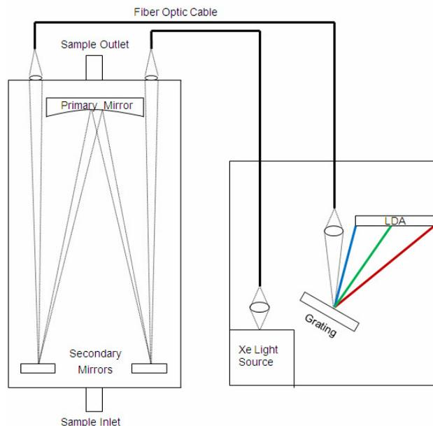
**Fig. 2.** A schematic of the benchtop AE-DOAS system. Light from the xenon lamp in the rack mountable spectrometer (shown on the right) is focused onto a fiber optic cable for transfer into the multi-pass gas cell (shown on the left). After a number of passes in the gas cell, the reflected light is focused onto a second fiber optic cable and detected by the spectrometer.
