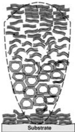
Figure 2: Variations of the microstructure in growth cones. Highly ordered layers at the top of the structure become more disordered closer to the carbon fiber (substrate) before resuming the highly ordered structure at the fiber surface. (Courtesy of Boris Reznik)
