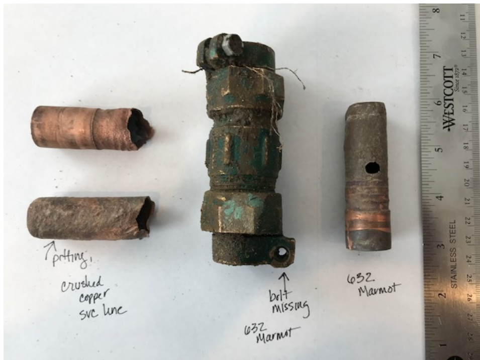
Corrosion and bad backfill materials will contribute to the failure of copper service lines.
