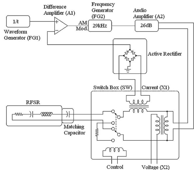
FIG. 3. Schematic of the control electronic circuit of the RFSR. An arbitrary waveform generator (FG1) sends a  $1/t$  ramp signal to a difference amplifier (A1). The amplifier outputs the signal difference between the  $1/t_{\text{tof}}$  signal and the rectified 29 kHz feedback signal driven by the spin rotator coil. Current and voltage signals are measured by ADCs for each neutron pulse (see Fig. 4).
