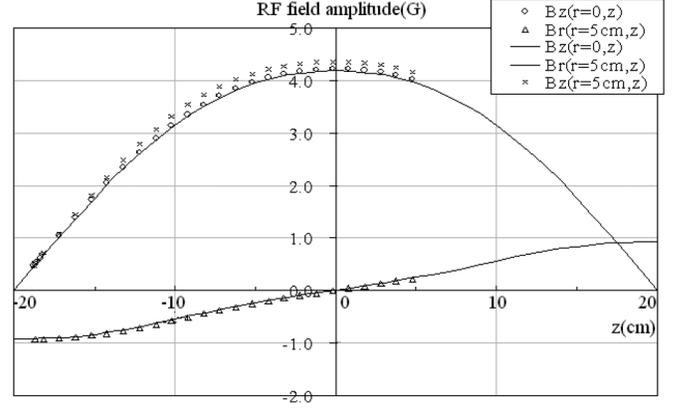
FIG. 5. Measured ( $\circ$ ,  $\times$ , and  $\triangle$ ) and calculated field components (solid lines) for  $B_z(r = 0 \text{ cm}, z)$ ,  $B_z(r = 5 \text{ cm}, z)$ , and  $B_r(r = 5 \text{ cm}, z)$  of the RFSR. The solenoid is 30 cm long and the RFSR, i.e., the rf field, is 40 cm long.
