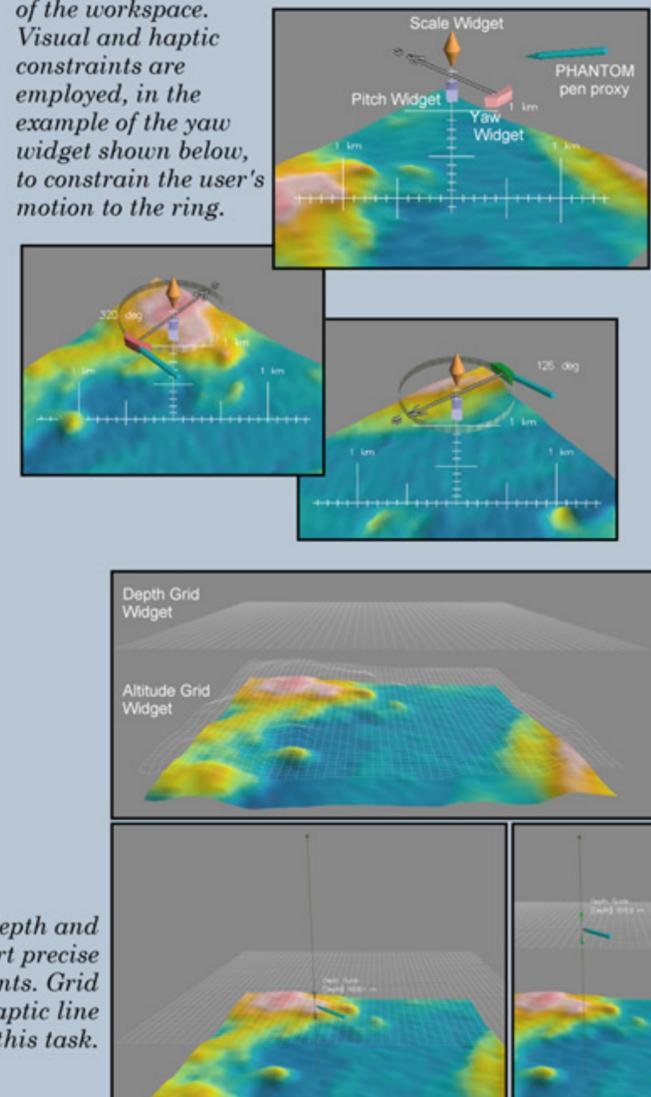
*Widgets such as the constant depth and constant altitude snap grids support precise placement of AUVs and path segments. Grid height can be adjusted directly; haptic line constraint forces guide the user in this task.*
