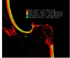
Figure 2. Bearing strength map created from geotechnical data collection at freshwater beach in the SWBTA.
