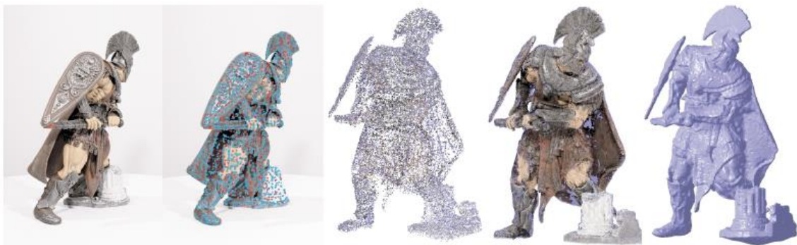
Figure 19. The overall approach of CMVS. From left to right: a sample input image; detected features; reconstructed patches after the initial matching; final patches after expansion and filtering; polygonal surface extracted from reconstructed patches.
