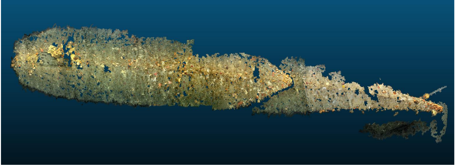
Figure 33. Full point cloud from all the images of top view sequence after bundle adjustment (Perspective 1).
