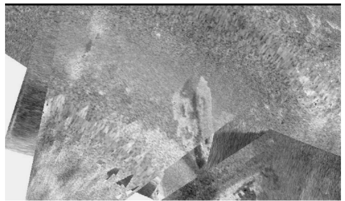
Figure 14 EA 400 Sidescan sonar mosaic, DTM used
