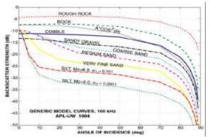
Figure 5 Relationships between acoustic backscatter and incidence angles for different sea bed materials at 100 kHz.
