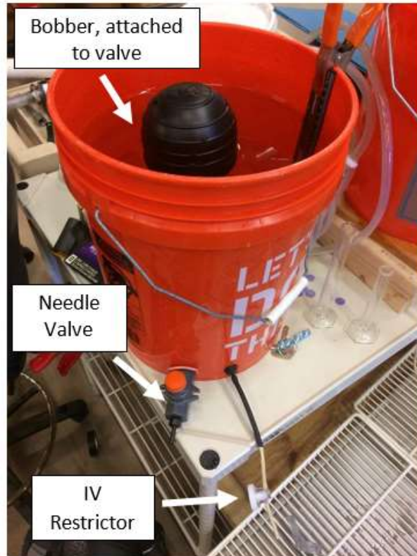
Figure 4: Photo of dosing reservoir with a bobber valve for water level control and IV restrictor and needle valve for outlet flow control.
